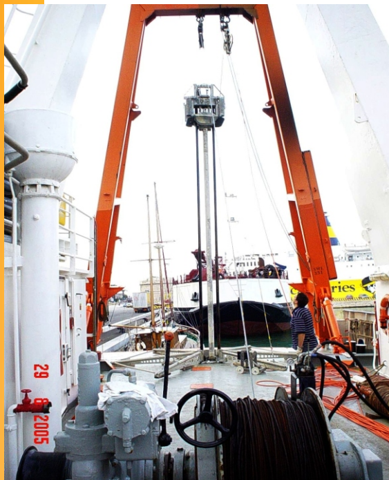
From the stern using the A-frame plus hoisting winch
