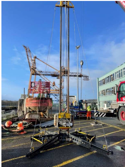
Figure 3-3 VC being assembled at Tivoli using a crane
